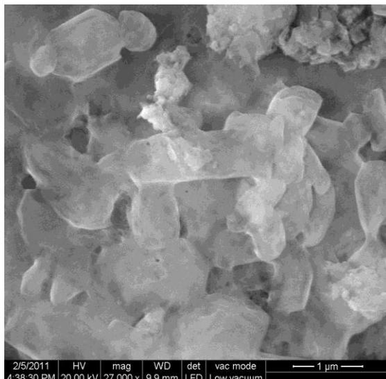
**Figure – 4(a) HR SEM micro graphs of pH 10.0 grown ZnO nano particles**
